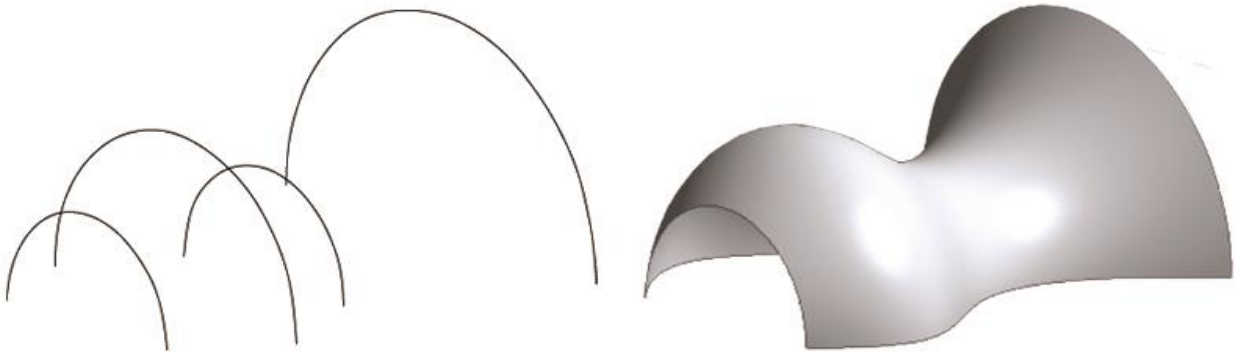
Figure 7: Process and development of instantiating a component onto a surface of a parametric system
