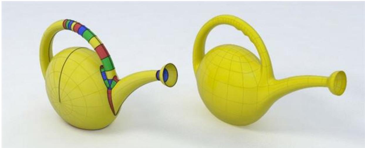
Creating the watering can model above (left) required many NURBS patches. This same model in T-Splines (right) is a single watertight surface.
