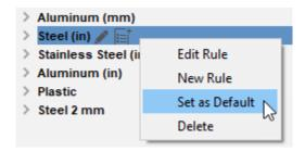
At any point in the design process, the active rule can be edited or replaced by another rule. Doing so will update all features in the model to the new active rule.
