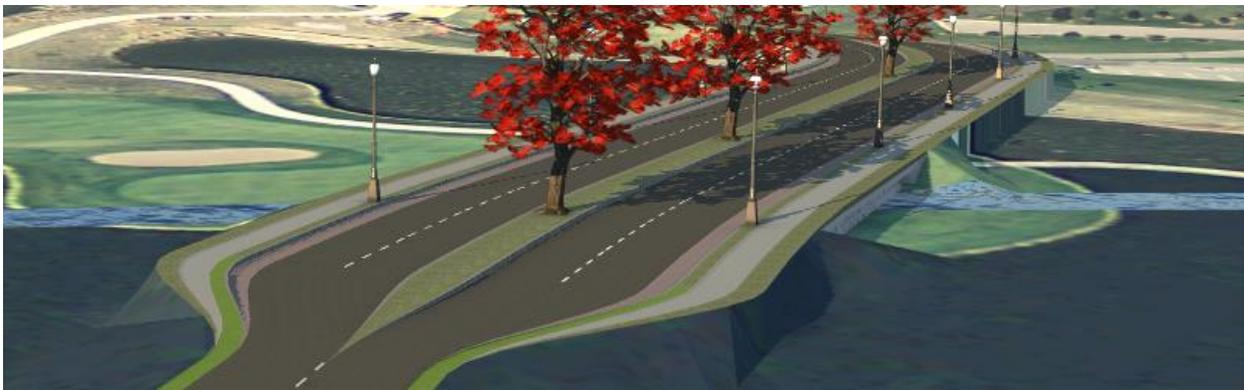
Another capability of design roads is that the tie-in slopes can be built according to a constant slope rather than a constant offset (that's what sketch roads do). This is much more representative of how roads are truly built.
