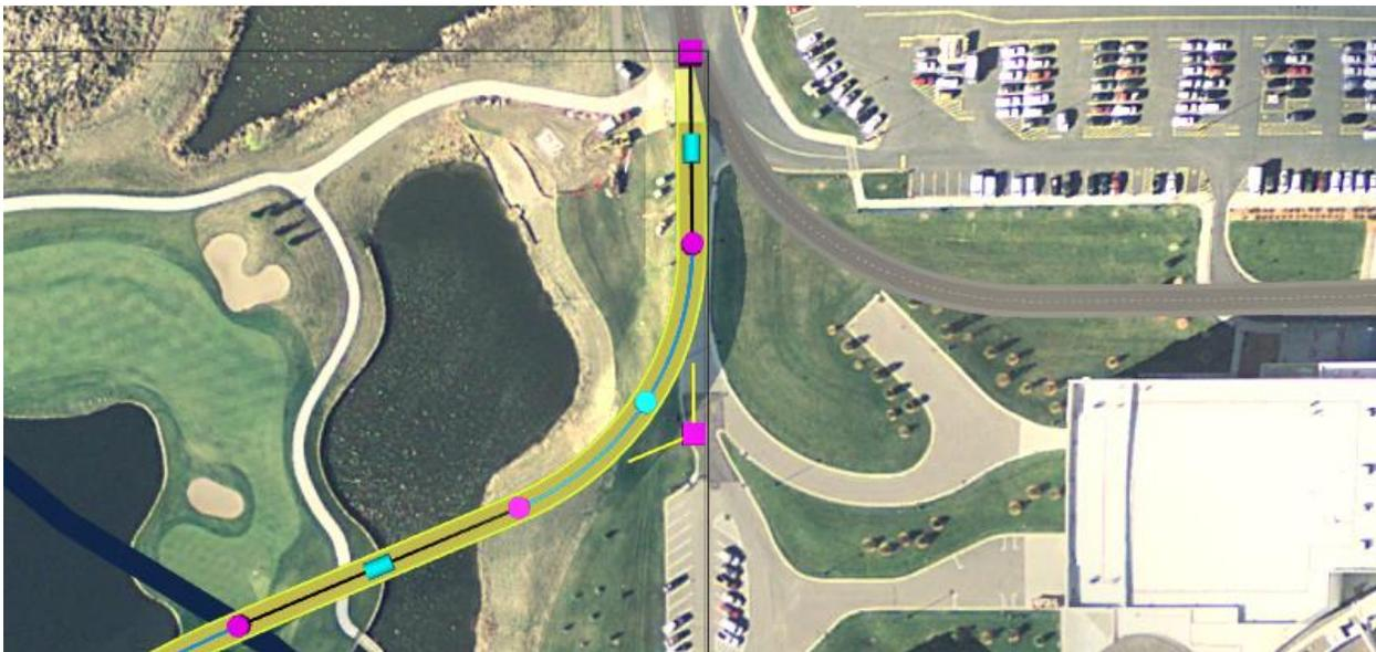
Something that Civil 3D can't even do, InfraWorks has gizmos (same idea as AutoCAD grips) located right on the road model, for both horizontal and vertical editing. When you change your view from top-down to more of an inclined view, the gizmos transform automatically and become PVI and vertical curve editing tools.
