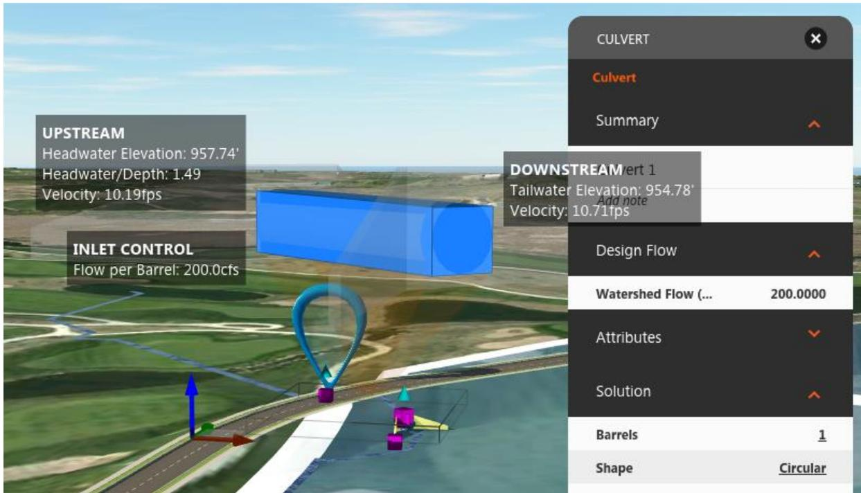
Of course you can manually create culverts and modify many aspects of their design including the layout as well as the shape, size, number of barrels, inlet configuration, and more.
