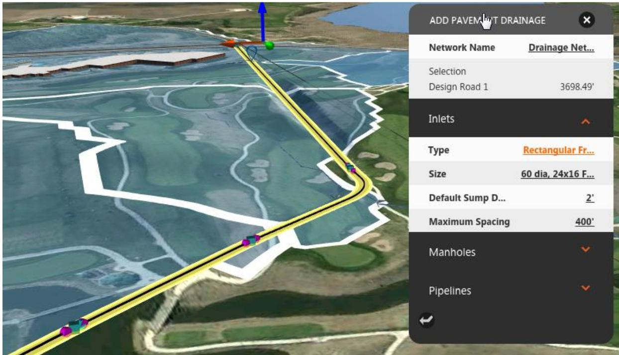
Or, you can do a combination of the two: let InfraWorks 360 lay out your drainage system automatically and then make changes, delete components, and add components to get the result you need.
