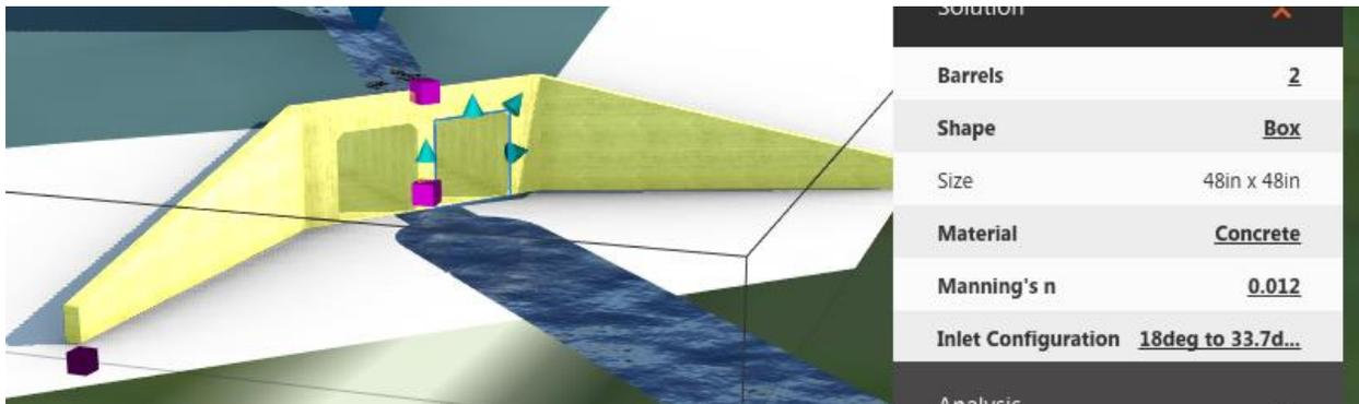
Pavement drainage is another feature set of Drainage Design for InfraWorks 360. You can create a system of inlets, pipes, and manholes for an entire design road or you can create the components individually using the tools on the drainage design toolbar.
