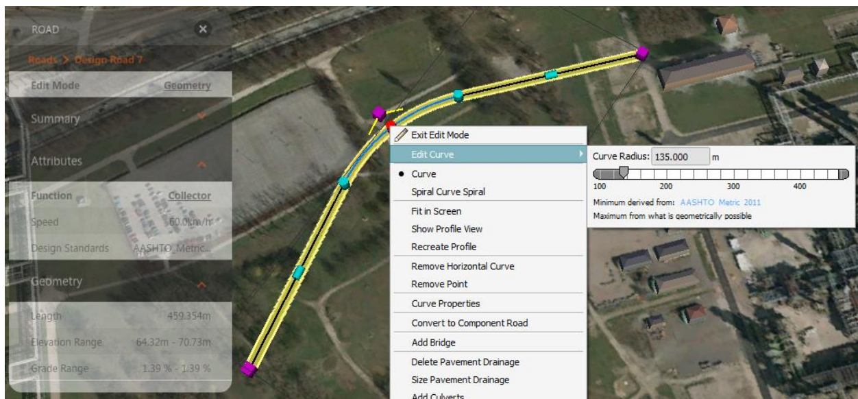
FIGURE 12: AASHTO 2011, COLLECTOR, MINIMUM CURVE RADIUS
