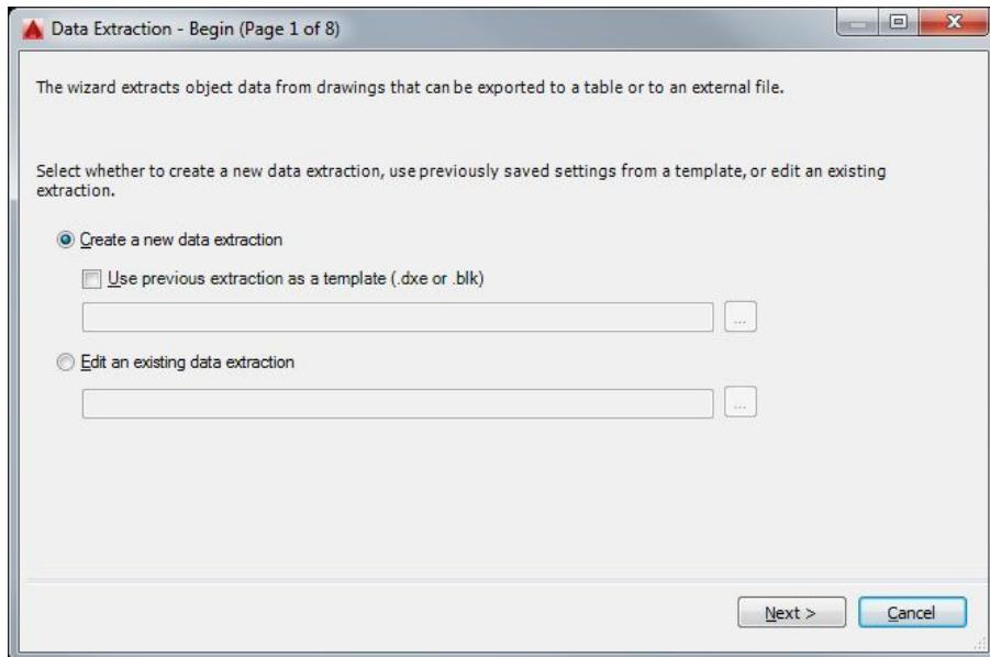
The first box allows you to create a new template or use and modify an old one.
