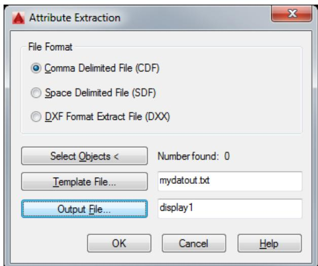
Using the ATTEXT command you can extract all the data in the drawing out to a txt file for uploading to Excel.
