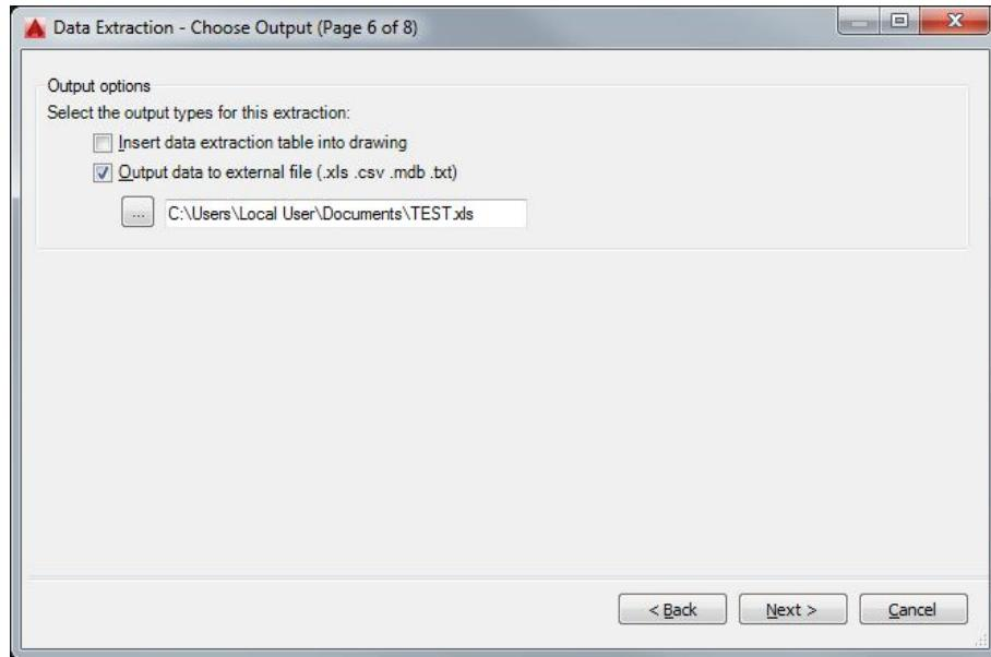
Six allows you to save the data in the drawing as a table (which will get you to box seven) or out of the drawing in one of the following formats xls, csv, mdb, or txt.
