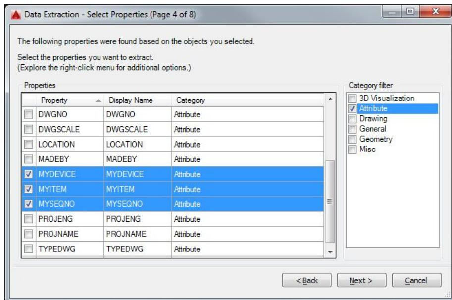
As you see there are more attributes than we are looking for in this drawing, the extraction takes all the entities in the drawing unless specified. So anything that is Layout as well as Model will show up in the list. Notice that by checking on and off different boxes you can select exactly what you need.
