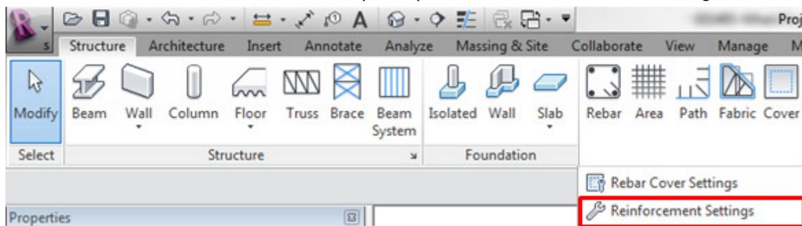
In the General Options, you can choose whether to host actual rebar elements within the area and path reinforcing similar to how beam systems and trusses host structural framing members, which you can then schedule and create rebar sets with. Or, you can choose to not host them, in which case you will only see representation of them when you cut a section view similar to previous versions.
