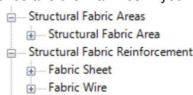
These are system families, and so the types must be created within the project environment. Expand these in the default Revit template to see the types already created.
