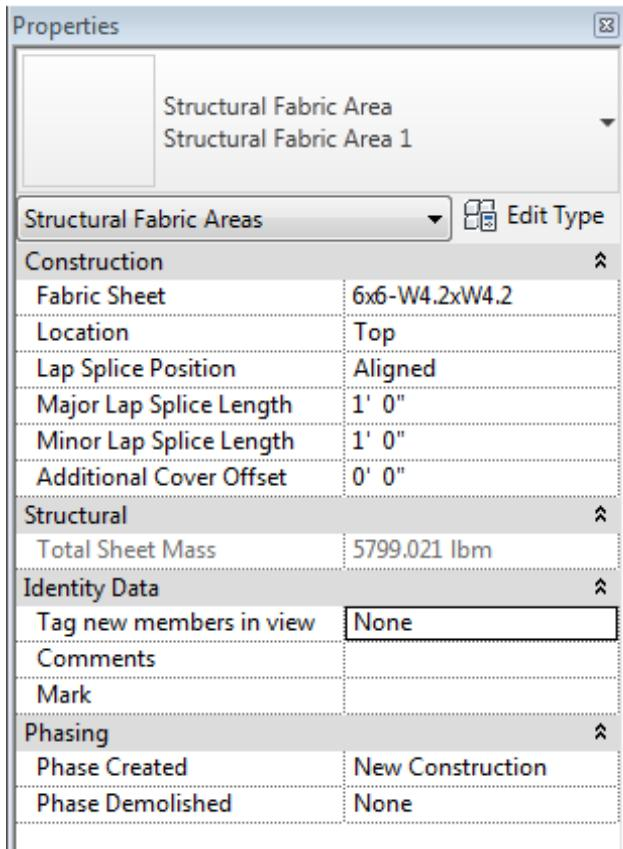
**Location:** Top or Bottom (Based upon your floor or wall's rebar cover settings) but can also include an amount in **Additional Cover Offset**
