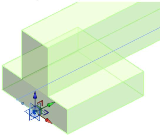
You can drag the point or use the coordinates icon to move the origin, and use the Rotate tool from the Modify ribbon to rotate it.
