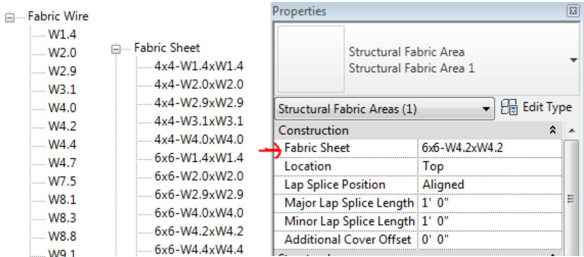
To Create a Structural Fabric Area ... Structure ribbon> Reinforcing panel > Fabric. Revit prompts you to Pick Structural Floor or Wall for Fabric Area Reinforcement. Then sketch the area to be reinforced.
