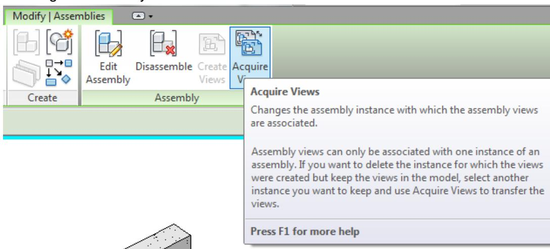
Always read the warnings when working with assemblies as new types can easily be created and views can be deleted or re-associated to a new assembly type.
