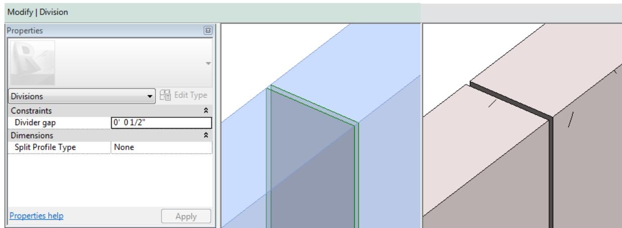
You can also select a Split Profile Type for elements/categories which always have parallel faces (walls, floors, roofs, slabs)... Three different profiles types come with the Revit 2013 content pack (Library>Profiles>Division Profiles):
