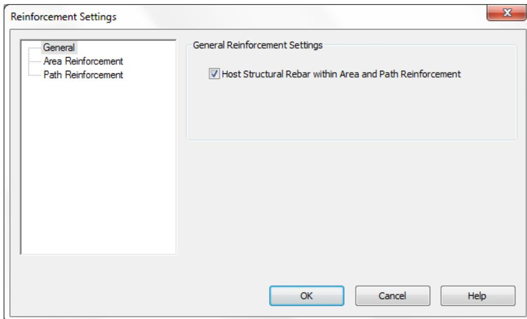
The default option is now to host the rebar. If you upgraded an older project to Revit '13 that already had area or path reinforcing placed, hosting will not be checked. This setting is applied to all area and path reinforcement elements in the entire project and cannot be changed after elements have been placed.
