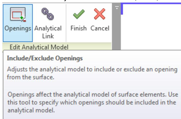
Note you cannot be working with only “Temporarily Display Only Analytical Model Categories” selected. You must have “Show Analytical Model Categories in this view” checked or have the analytical categories checked on in Visibility Graphics for the opening tool to work properly.
