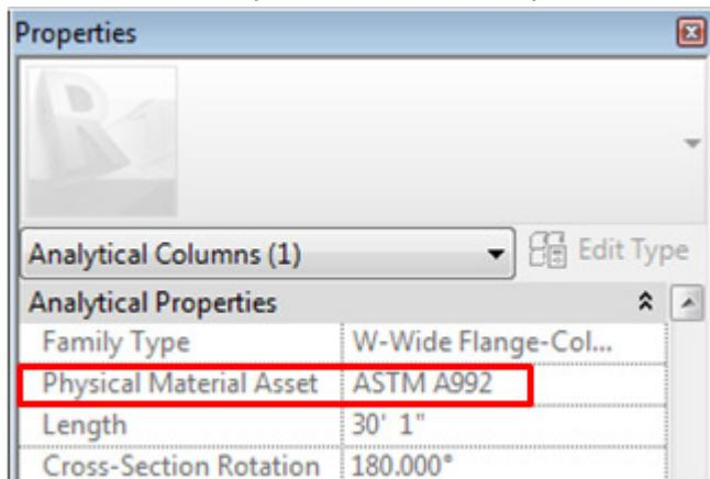
The physical material asset includes the thermal, Mechanical, and Strength properties of the material that can be exported to your analysis software. This information is being pulled directly from the physical model's Structural Material.
