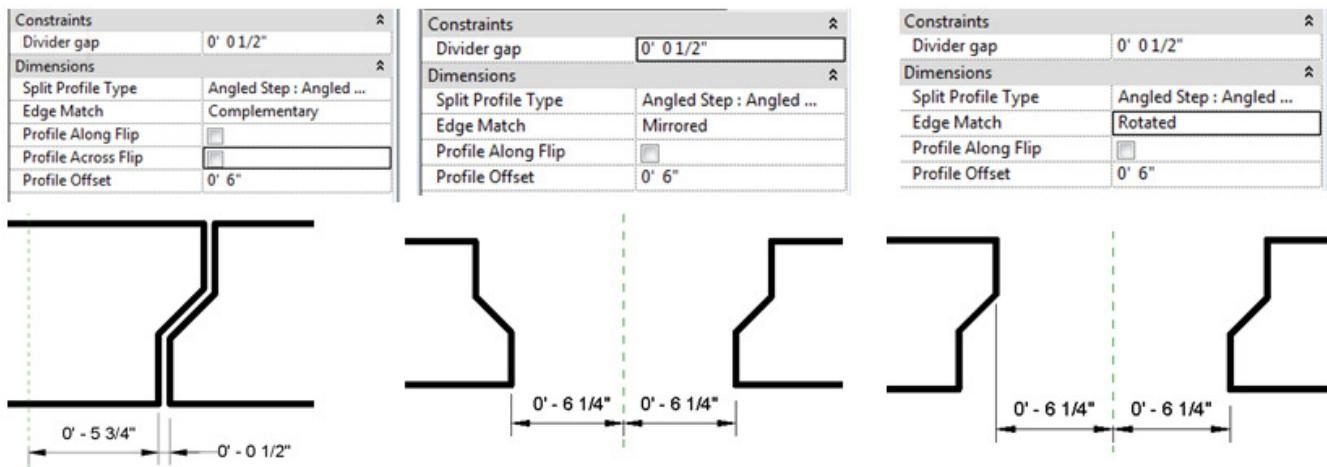
As you can see for the Mirrored and Rotated profiles it probably makes more sense to use either the Divider Gap distance OR the Profile Offset distance, but not both.
