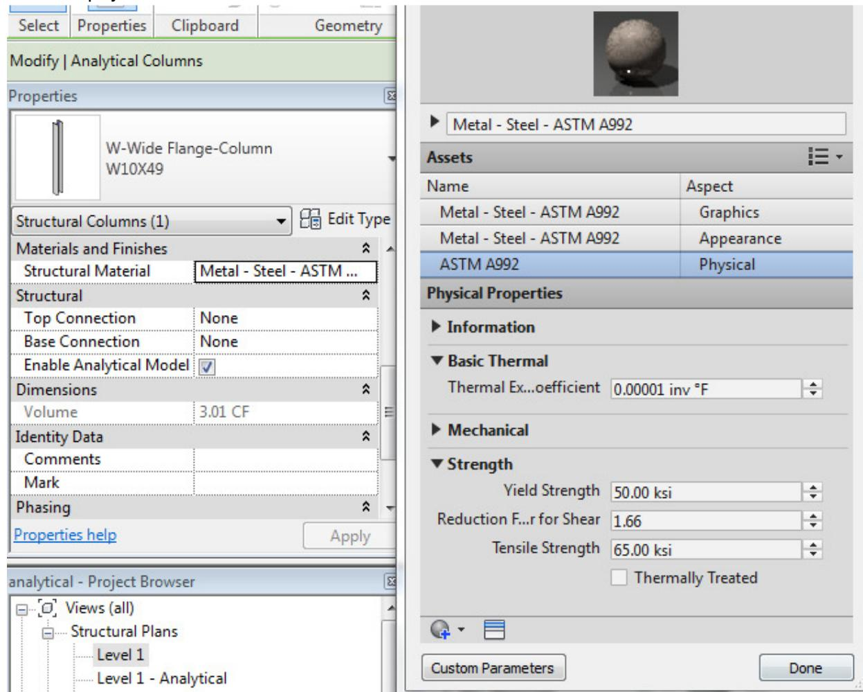
To ensure that the Physical Material properties are exported out to your analytical software you can turn on the Valid Physical Material Asset check.
