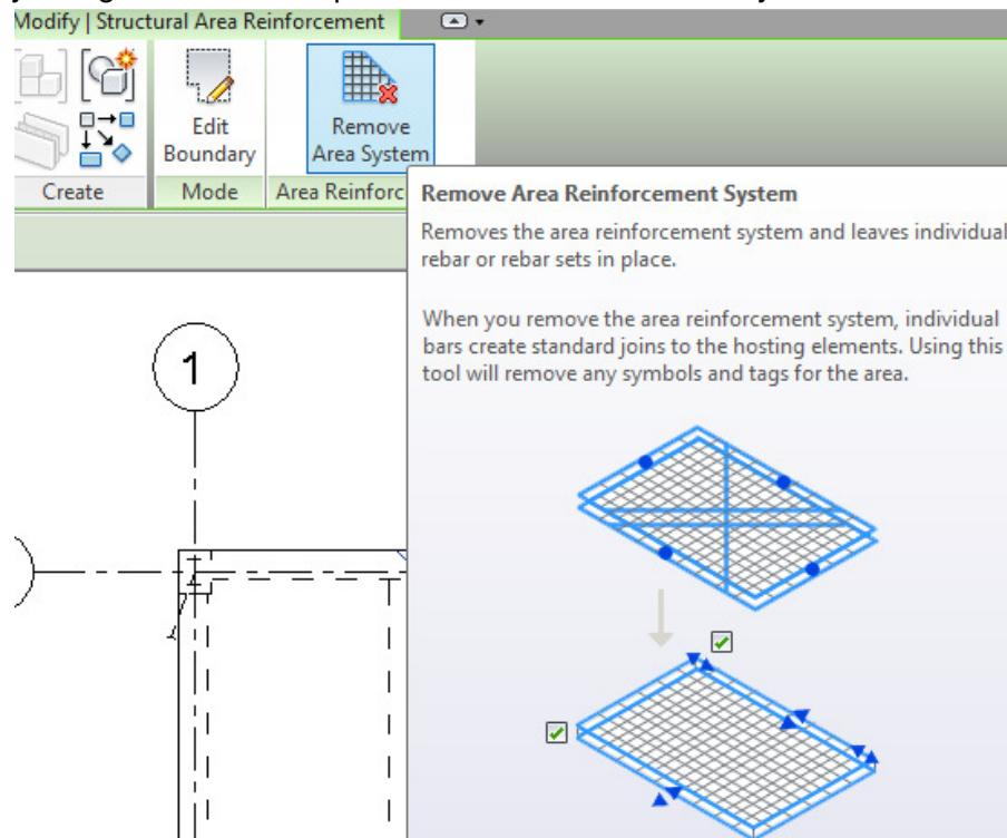
When you remove the Area or Path reinforcing system, all rebar sets will be shown individually, as if you had placed them with the Rebar tool instead of the Area/Path tool. You can then modify each set's size, spacing, and layout individually.
