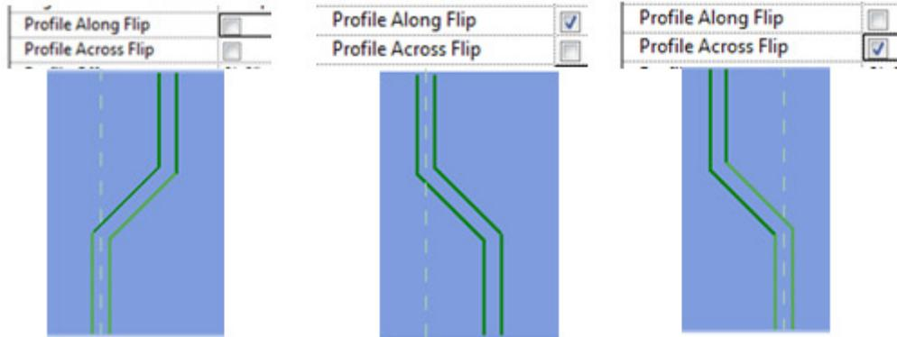
The profile offset is the distance the profiles are offset from the dividing line. Remember to also take into account the distance you set for the divider gap which is offset about the center of the division line. For example, if I set the divider gap to  $\frac{1}{2}$ " and the Profile offset to 6" this is how my divisions would look:
