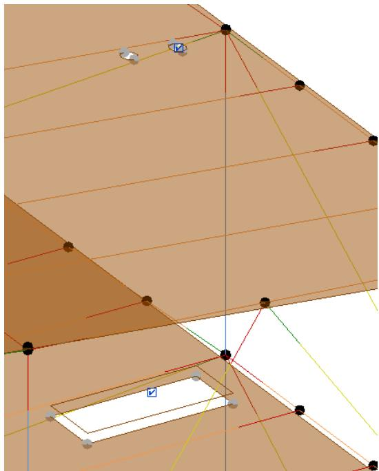
When I click the Openings tool, a check mark is shown at each opening location. Once I uncheck it, the opening is filled in.
