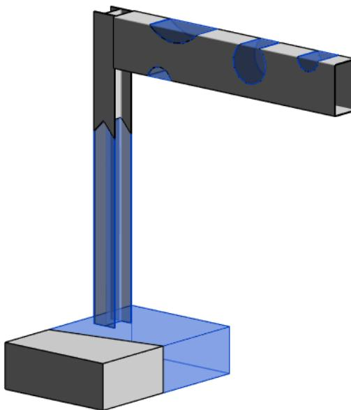
Revit will remember your edits to the parts when switching between types of the same family (i.e. HSS12 to HSS10) however will only remember that parts were created (resetting their shape) when switching types to a different family (ie HSS to W-Flange).
