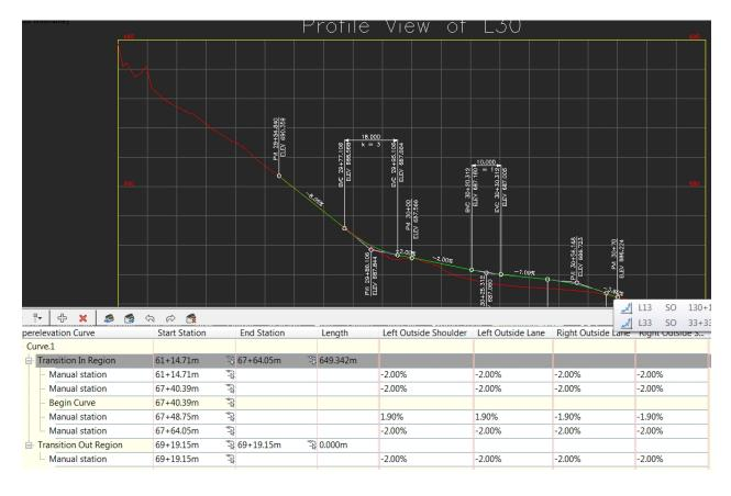
The L30 profile is 2% across the intersection but the two alignments are not perpendicular. This skew means that the slopes across the L67 lanes have to be something less than 2%
