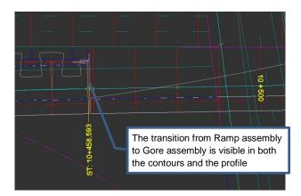
I have edited the design profile and temporarily added a three point curve which provides a grade for the ramp at the tie in point. With this information I can finish editing the design profile and rebuild the corridor to complete this ramp.
