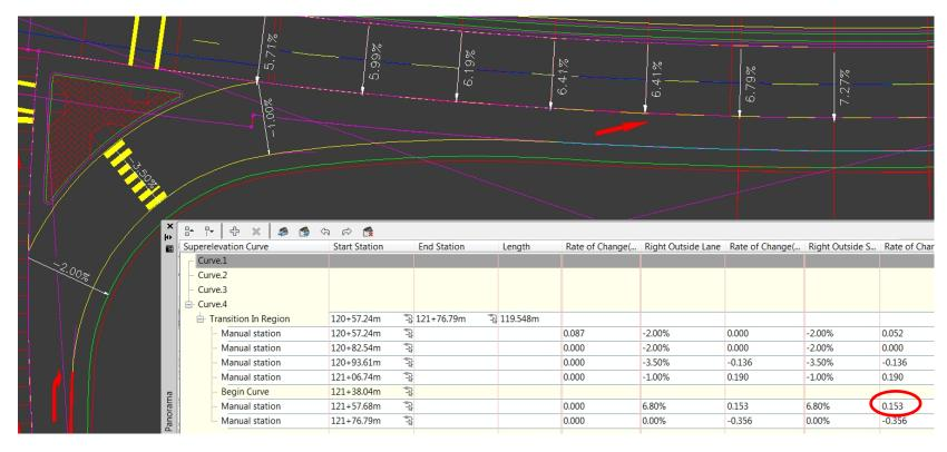
The solution here was to select a suitable Rate of Change in the superelevation parameters, and use that to calculate the point where the crossfall of the turn lane would match that of the highway.
