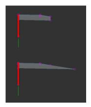
LinkVertical subassemblies with the Omit Link option turned on are inserted at the red lines to allow these assemblies to shift up or down from their insertion point to match the elevation of the targeted featureline.
