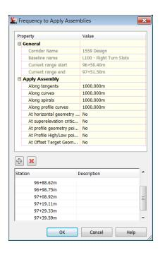
The second problem comes from the fact that the top and bottom of the road structure isn't parallel. The ShoulderExtendAll subassemblies being used here all have the same default thickness at their inside edge. The only way that I've been able to fix them is using the corridor view editor. Measure the thickness of the subbase material at the outside edge of each subassembly, and apply that to the inside thickness of the next sub.
