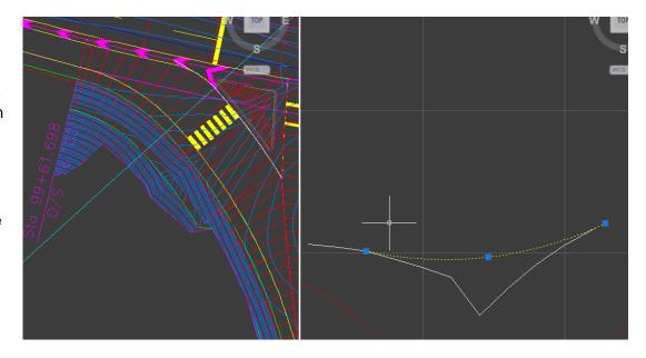
The deceleration lane from the west has a similar issue with transitioning the crossfall as we've already seen on the east side acceleration lane. I have already set up the superelevation parameters – matching the existing lane slope at the start of the turn lane and the -2% slope of the turn slot at the other end. Create another baseline for the L100 – Right Turn Slot alignment, add a region and assign targets.
