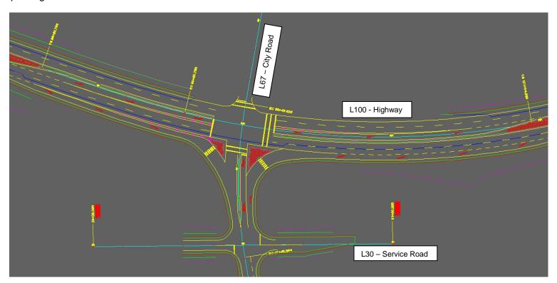
All of the 2d linework in the Design Base 4 – 1 drawing has already been drawn to suit the design standards of the Ministry of Transport, and the City. The geometry of the intersections has been checked with turn simulation software to confirm that fuel trucks can get in and out of the gas station, and other trucks can access the industrial development.
