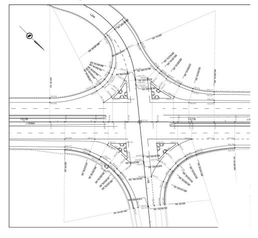
When the wizard calculates the curb return profile it uses a single value for the crossfall from each of the mainline alignments. There is no option for crossfall transitions along the incoming and outgoing lanes.
