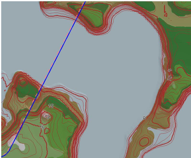
Our result is an extremely large lightweight surface with contours and labels that we can quickly use for analysis, creating profiles, sections...
