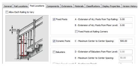
d. Set the height and width of the handrail approximately for a single rail.
