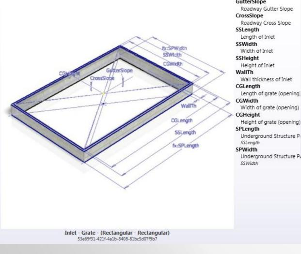
GutterSlope Roadway Gutter Slope CrossSlope Roadway Cross Slope SSLength Length of Inlet SSWidth Width of Inlet SSHeight Height of Inlet
