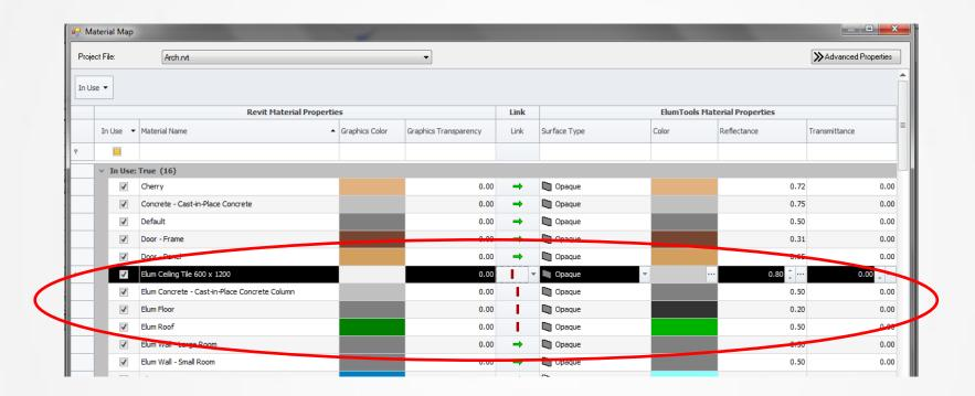
4. For the purpose of this example we have entered the default settings of ceiling 0.8, walls/columns 0.5 and floors as 0.2 reflectance.
