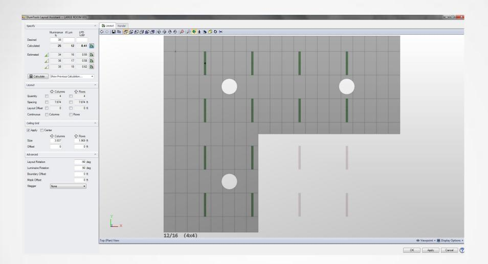
Once you have calculated and happy with the result. You can now select **OK** which will past the desired lighting layout into the Revit Model. Now you can simple calculate using the regular Elumtools method allowing the calculation points to appear and your schedules to be populated.
