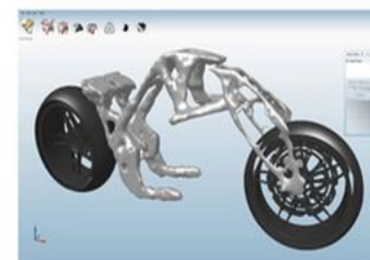
Altair design software produces ideal shapes for vehicle parts like this motorcycle frame. Altair
